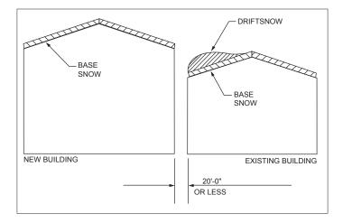
Placing a new taller building adjacent to an existing building can result in snow drift loads on the existing building that were not considered in the original design. The new snow drift load could cause the original building to collapse. When adding a new building within 20 feet of an existing building, the existing building should be checked for potential additional loads and reinforced if necessary.
